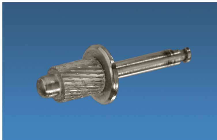
Fig. 2 The newly developed step cutter to create the circular step in the mandibular stumps
