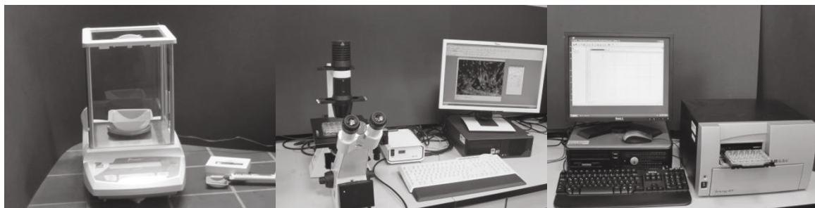
Figure 1 Analytical balance (Pioneer PA64, Ohaus, Pine Brook, USA), left; inverted fluorescence microscope (Axiovert 40C/Carl Zeiss, Göttingen, Germany), middle; fluorescence/luminescence reader (Synergy HT-Reader, Biotek, Winooski, VT, USA), right.
