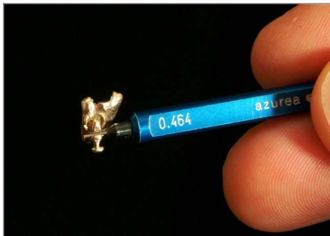
Figure 4 End of measurement. Measurement of slot precision ended when the bracket was attached to the pin gauge by friction.
