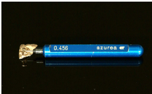
Figure 3 Start of measurement. Start of measurement of slot precision by insertion of the smallest pin gauge with a dimension of 0.456 mm (0.01795 Inch).
