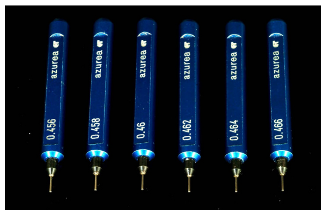
Figure 2 Pin gauges. Precision pin gauges tapered in increments of 0.002 mm (0.00008 inch).
